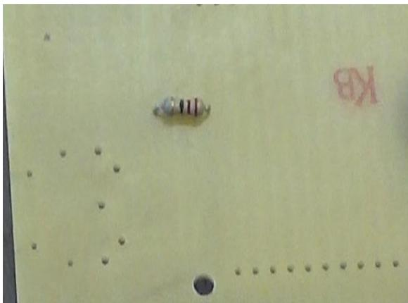
The single resistor goes in the two holes adjacent to the holes for the Midi Socket as shown here. It doesn't matter which way round it goes.
